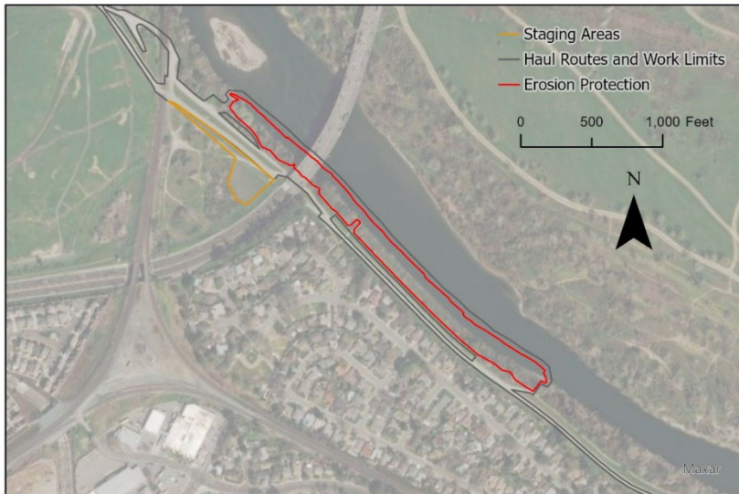
Figure 1- 4 Bank Protection and Launchable Toe Footprint
