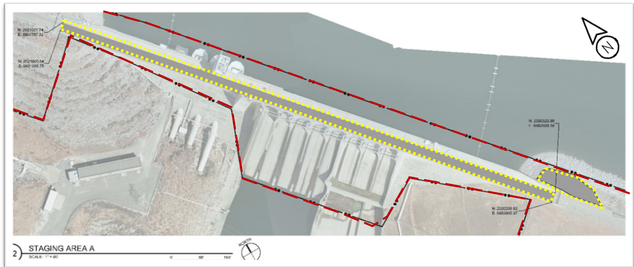
Figure 2-17. Folsom Main Dam Tainter gate refinements: Limits of construction (dashed lines) and construction staging areas (dotted lines).
