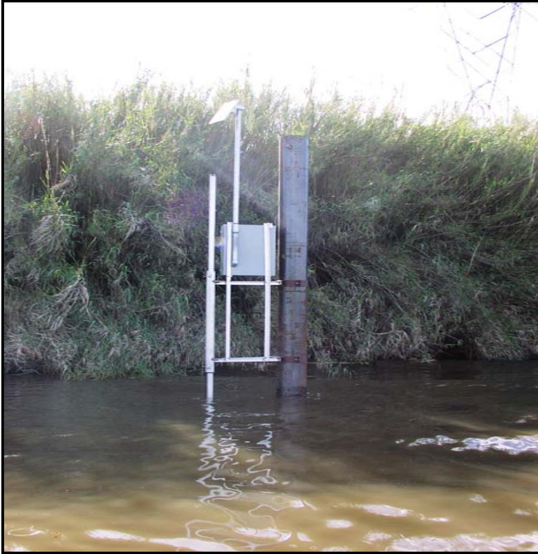
FIGURE 2: Typical Acoustic Doppler Current Profiler Monitoring Station.
