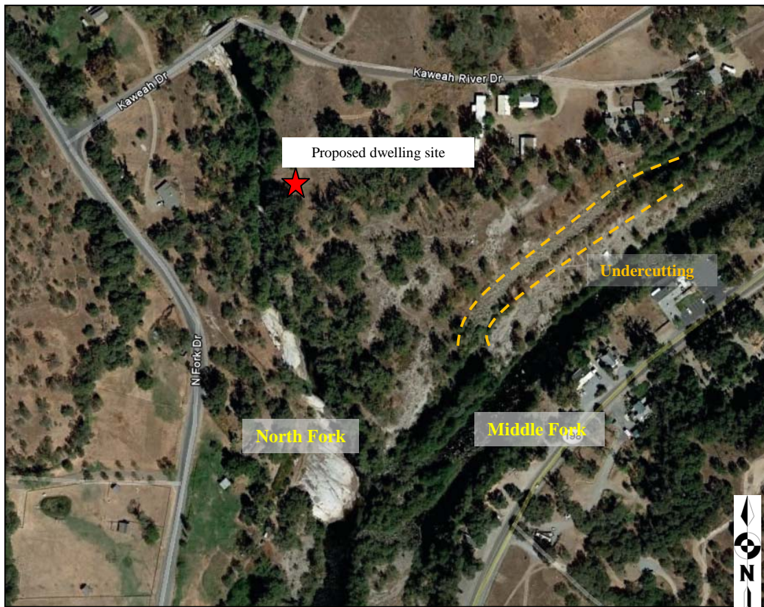
Figure 5. Aerial view of project location showing undercutting on west bank of Middle Fork.
