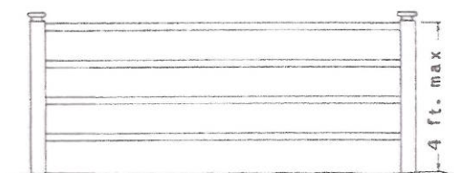
WOOD POSTS AND RAIL FENCE SPACING OF POSTS 8.0 FT. MINIMUM.
