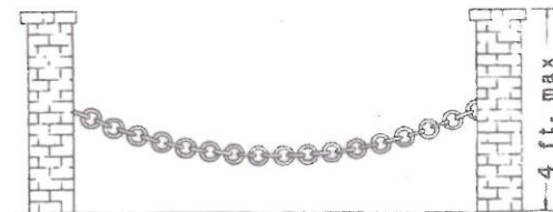
BRICK PIERS AND CHAIN FENCE MATERIAL FOR PIERS OPTIONAL—BRICK, CUT STONE, RUBBLE OR CONCRETE. SPACING OF PIERS 8.0 FT. MINIMUM.
