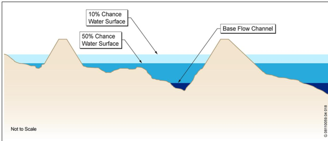
**Figure 2-2. Water Surface Elevations by Floodplain Inundation Potential**
