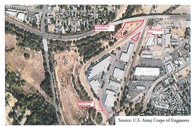
Figure 2. Proposed staging areas for the Natomas East Main Drain Canal North Extension, Sacramento County, California.
