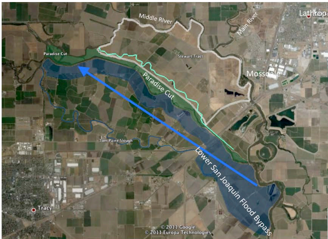
Figure 1. Expanding Paradise Cut (green) with a Lower San Joaquin Flood Bypass (blue) will route floodwaters away from urban areas in Lathrop and Stockton along the mainstem of the San Joaquin River. Blue arrow shows direction of flow and orientation of expanded bypass to the south. Light green shows widening of Paradise Cut using levee setbacks on River Islands.
