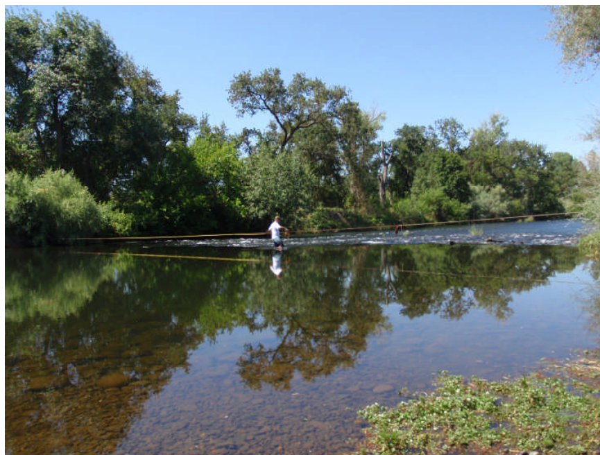
Figure 3. Technician stretching measuring tape across a river channel.
