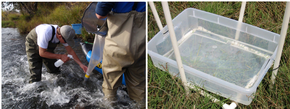
Figure 4. Biologists using Hess Stream Sampler to collect benthic macroinvertebrates in the Stanislaus River (left) and a typical fallout trap (right).
